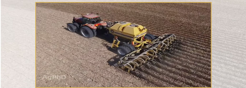
Figure 12. Soils Using Strip-Tillage Machine.
