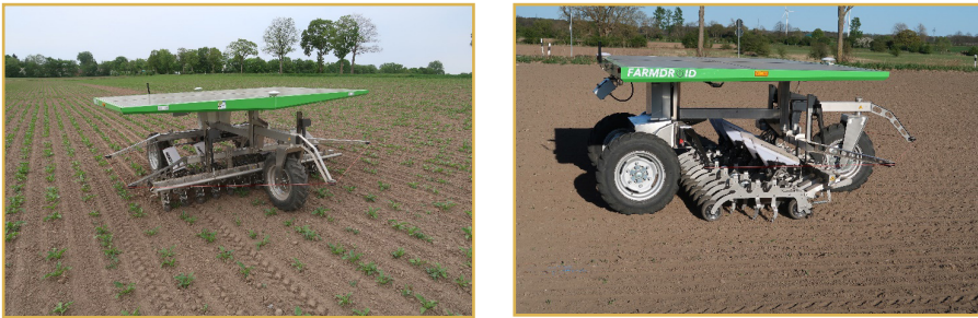
Figure 102. Solar powered autonomous field robot
