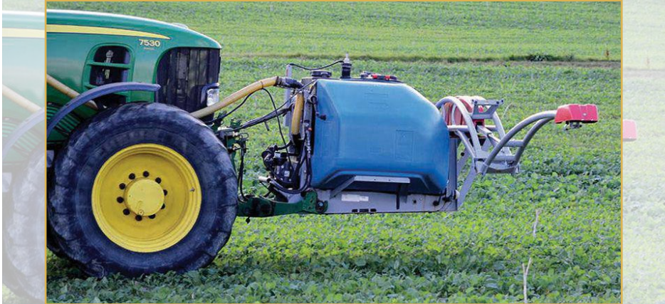
Figure 92. Optical sensors on the front of the tractor
