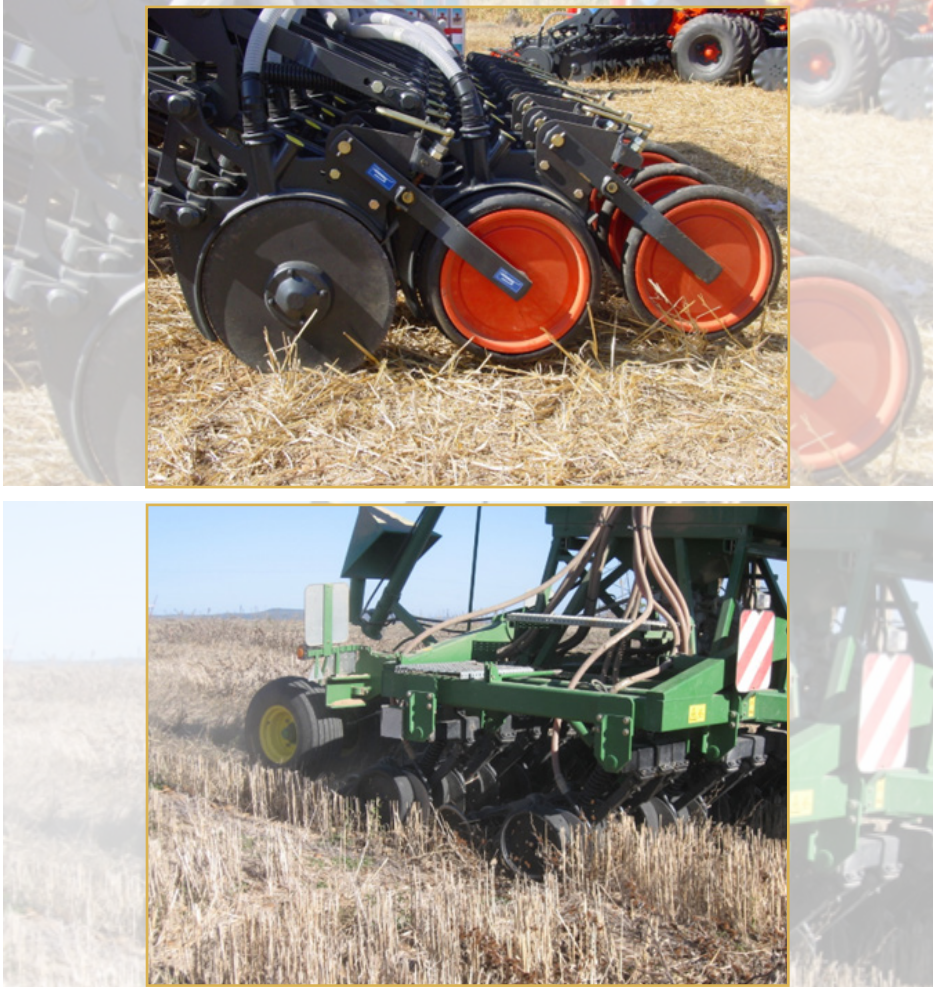
Figure 3 & 4. Disc coulters Direct Seeder.
