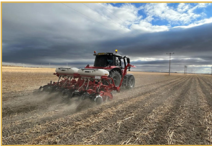
Figure 18. Strip-Tillage Machine with 6 and 4 rows.
