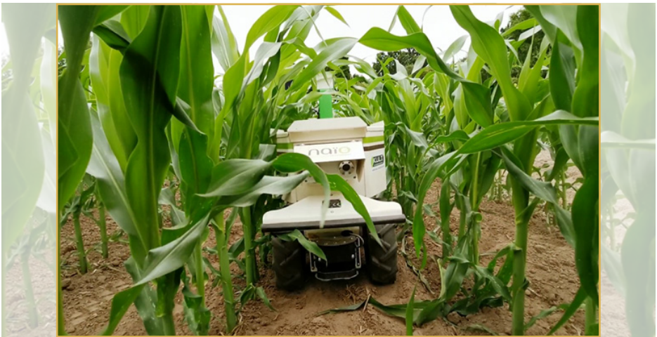
Figure 100. Small Weeding Robot between Maize rows
