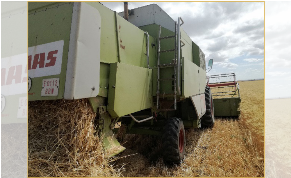
Figure 32. Harvester expelling the straw.
