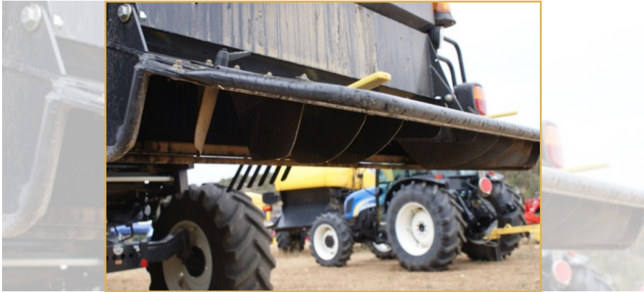
Figure 34. Rear deflector detail
