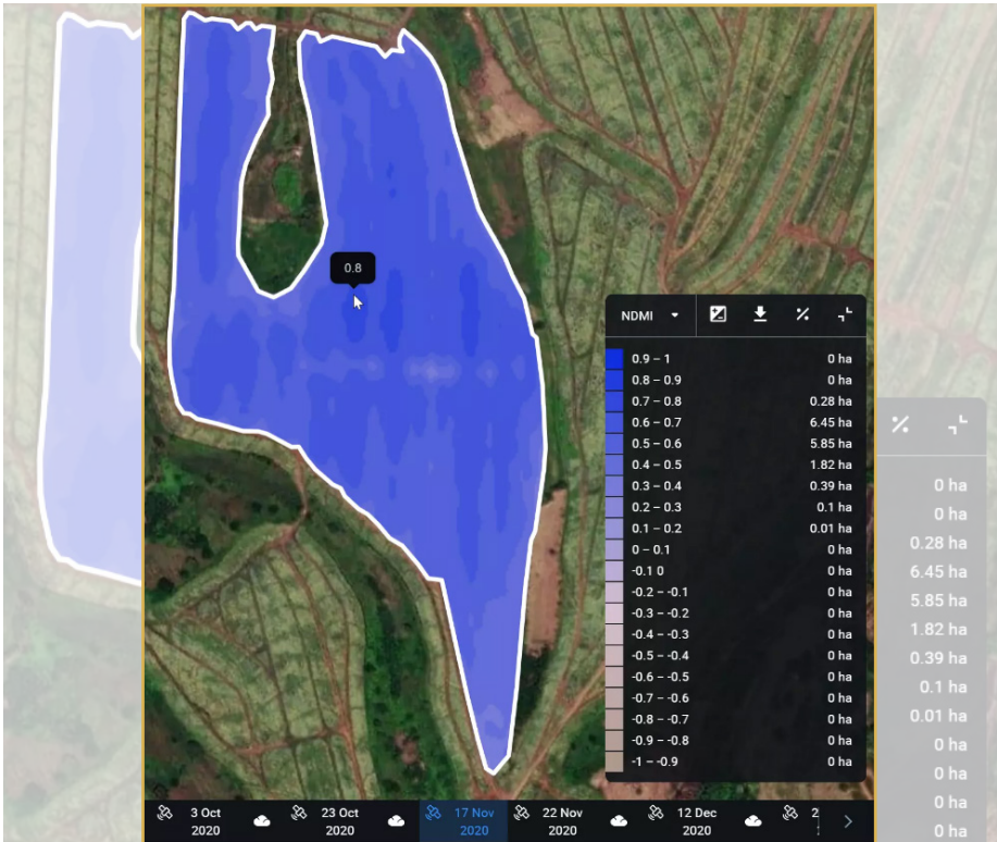
Figure 114. Example of field with ndmi index calculated on it.
