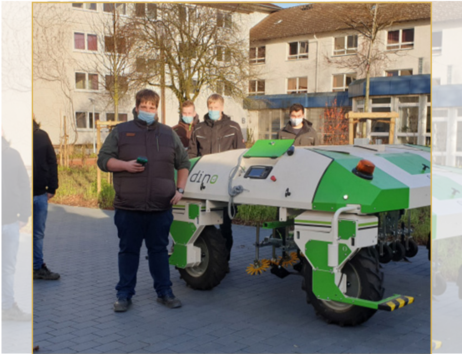
Figure 101. Batterie powered autonomous weeding robot
