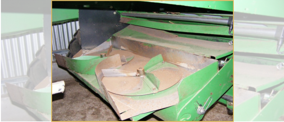
Figure 33. Detailed system spreader of residues in the cereal harvester
