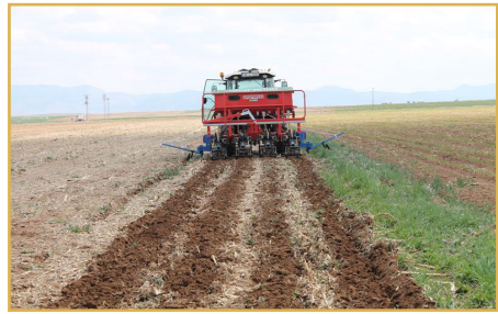
Figure 18. Strip-Tillage Machine with 6 and 4 rows.
