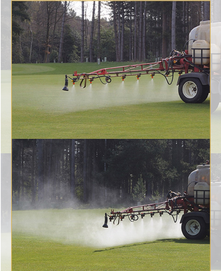
Figure 107. Comparison in the use of standard and anti-drift nozzles
